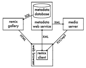
Figure 1. Components of the International Remix system.
